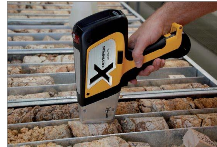
Analysing geological drill cores (left); hydrogeological maps of aquifer qh in Quy Nhon (centre); pXRF analyser (right).
